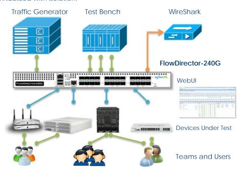
Additionally the FlowDirector provides total visibility into the network without impacting DUTs or test setup. The on-demand tapping capability has been proven to be useful for engineers and administrators to obtain information and diagnose the root cause.
